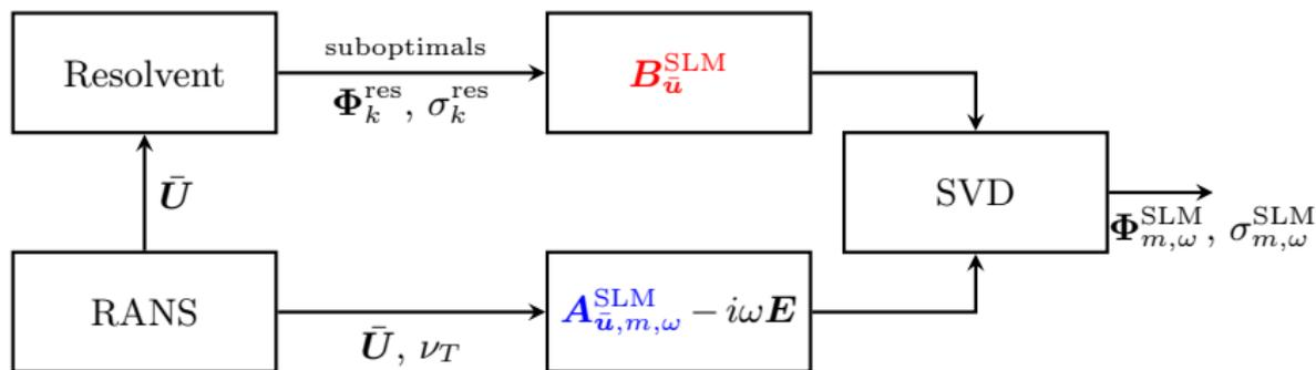
Figure: Schematic representation of the SLM procedure.
