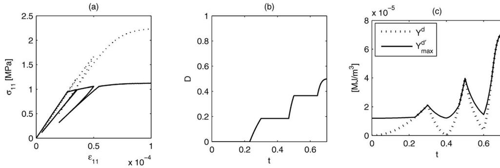
**Fig. 5.** Uniaxial behavior of an endochronic plasticity model with damage (Definition 1): (a) the stress–strain evolution. The dotted line indicates the effective stress  $\sigma_{11}/(1-D)$ ; (b) damage evolution; and (c) see Fig. 3(c).
