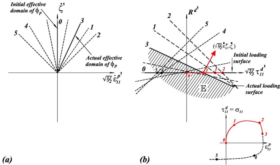
**Fig. 4.** Endochronic model with damage in the uniaxial stress regime. (a) Several configurations of the effective domain  $D$  of the pseudopotential  $\phi_p$ . (b) Corresponding configurations of the loading domain  $E$ , associated with the loading function  $f_p$ . The actual stress point always occurs at  $R^{d'} = R^d = 0$  and, at this point, the flows  $\dot{\epsilon}^p$  and  $\dot{\zeta}$  are defined by the normality condition.
