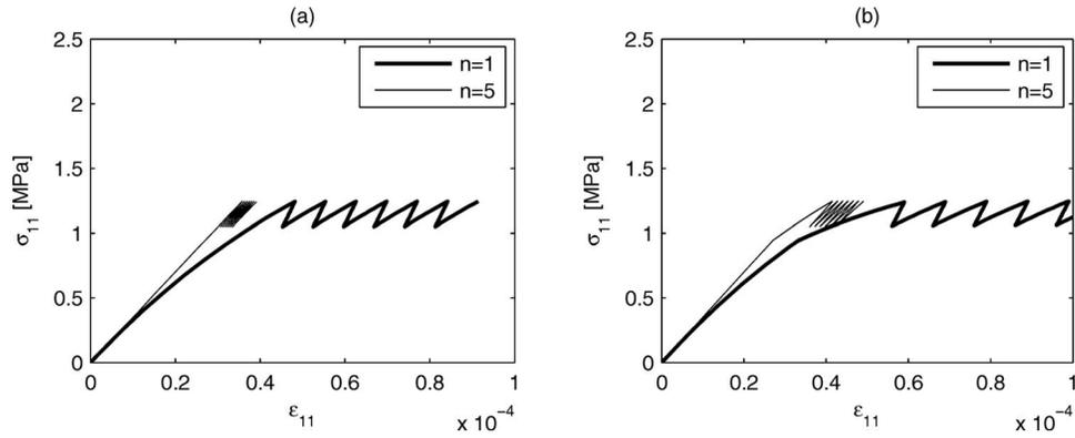
**Fig. 7.** Strain accumulation, uniaxial behavior with stress varying between 1.05 and 1.24 MPa. (a) Endochronic model without damage, with the intrinsic time (4). (b) Endochronic model with damage, with the intrinsic time (9) and the damage evolution given by Eqs. (27) and (33), with  $r_0=0.000012$  and  $s=6$ .
