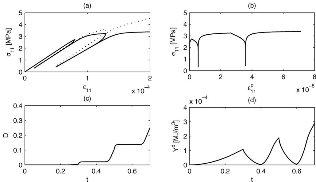
**Fig. 6.** Uniaxial behavior of an endochronic plasticity model with damage (Definition 2). (a) The stress–strain evolution. The dotted line indicates the effective stress  $\sigma_{11}/(1-D)$ . (b) The stress as function of the plastic strain. Observe that the plastic strain increases during unloading phases. (c) The damage evolution, with damage slightly increasing also during unloading phases. (d) Evolution of  $Y^d$  versus time.
