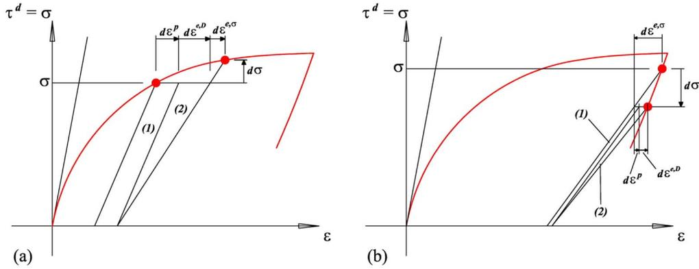
**Fig. 2.** Increment  $de_p$  of the energy dissipated by plastic strain (1) and the increment  $de_D$  of the energy dissipated by damage (2). The increments of the elastic and plastic strain as well as of the stress are also schematically illustrated for (a) the loading phase and (b) the unloading phase.
