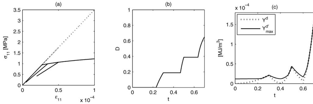
**Fig. 3.** Elastic with damage model. Uniaxial behavior. (a) The stress–strain evolution. The dotted line indicates the effective stress  $\sigma_{11}/(1-D)$ . (b) The damage evolution, with the damage increasing only during loading phases. (c) Time evolution of  $Y^d$ , i.e., the actual value of the thermodynamic force  $Y^d$ , and of  $Y^d_{\max}$ , i.e., the upper bound of  $Y^d$  defined in Eq. (29).
