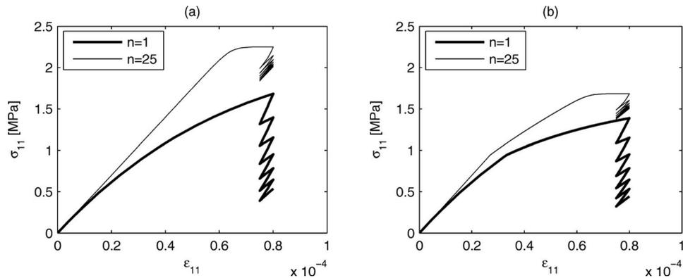
**Fig. 8.** Stress relaxation, uniaxial behavior with strain varying between 0.000075 and 0.00008. Endochronic model (a) without damage and (b) with damage, with the same damage parameters as in Fig. 7(b).
